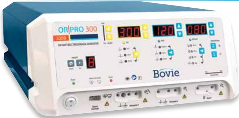
Bovie introduces the Aaron® OR|PRO 300 Electrosurgical Generator. The system was designed in conjunction with OR clinicians to provide a safe, user-friendly generator to meet all operating room procedure performance demands. This innovative energy-based device offers 13 modes of surgical energy delivery. Special modalities include the advanced Bovie Bipolar, Auto Bipolar options, and special Laparoscopic modes.
